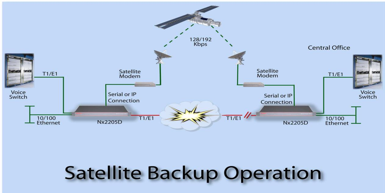
Other benefits provided by the Nx2205D include fractional backup (using proportionally less bandwidth), anti-bounce for channel/circuits prone to brownouts, activity logging and alarming.
